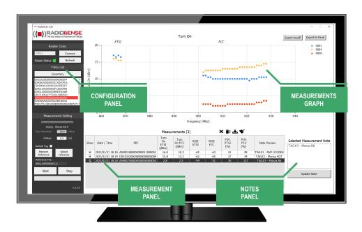
\*TTSLab is the processing software that activates the interrogation of the environment and lists all the tags detected in the surroundings with the corresponding EPC code, measuring the respective ignition powers in real time. The data is represented through a simple and intuitive graphic interface.
